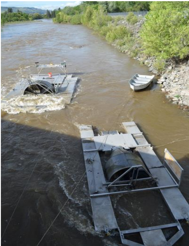
Figure 3. 2.4-m (left) and 1.5-m (right) traps fishing in the Okanogan River. The boat is used by technicians to access the 2.4-m trap. Photo by CCT.
