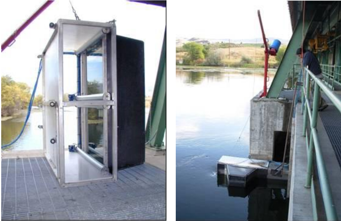
Figure 4. Photographs of Zosel Dam west bank video chute array prior to (left) and during deployment.
