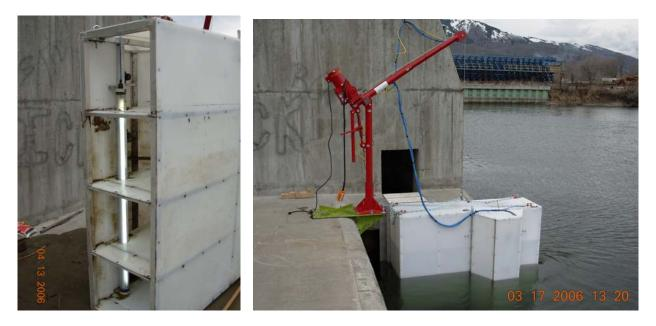
Figure 4. Photographs of Zosel Dam east bank video chute array prior to (left) and during deployment.
