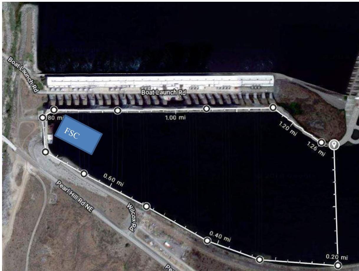
Figure 7-7. Concept for possible Location of Chief Joseph FSC (blue box). White line denotes powerhouse effective forebay area. Total effective forebay area is 51 acres.
