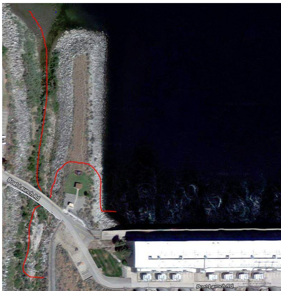
Figure 7-10. Aerial view of possible adult fish ladder at Foster Creek with secondary entrance in tailrace. Line in red shows site of adult fish ladder and entrances. Facility would be like that shown in Figure 7-9.
