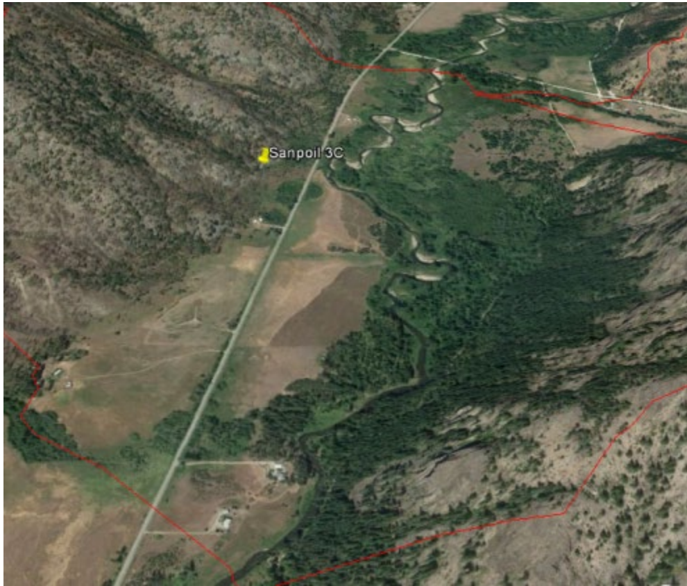
Figure B-44. Overview of Sanpoil 3C reach. Note State Route 21 on the west side of the valley and the gravel road along the east side of the valley, with single-thread channel meandering across the valley. Red lines indicate the extent of lands draining to the study reach.
