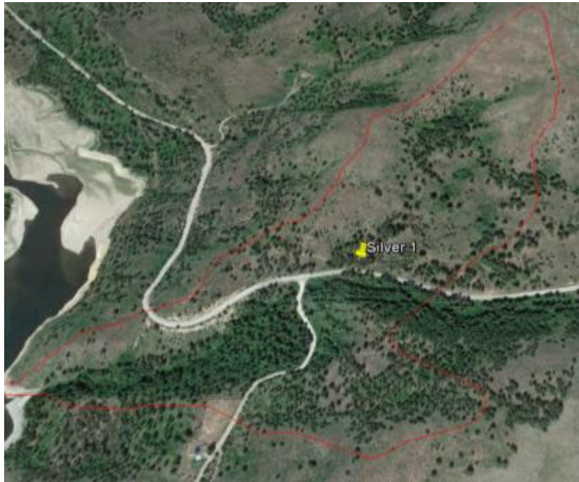
Figure B-56. Overview of Silver 1 reach. The stream confluence with the Sanpoil Arm is in the lower left portion of the image. The red line indicates lands draining to the study reach.
