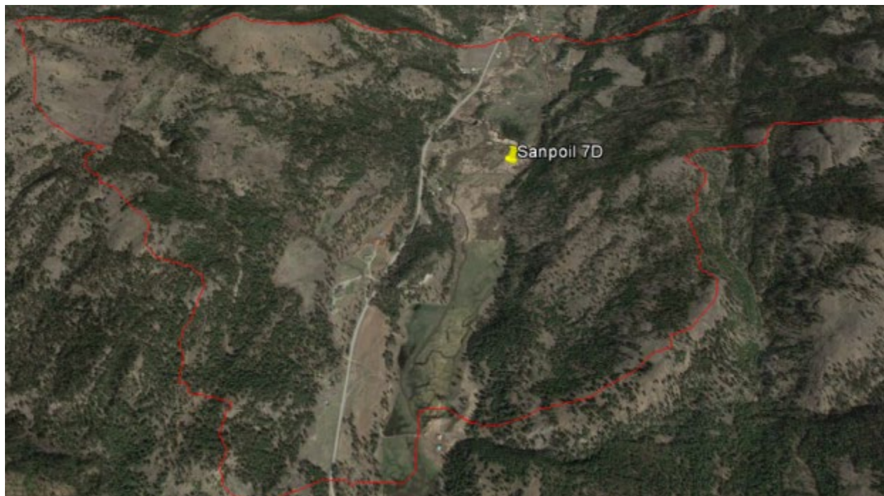
Figure B-7. Overview of Sanpoil 7D reach. This reach is almost entirely in agricultural production. There is virtually no shrub or tree riparian cover. Red lines indicate the boundary of upslope lands draining to the reach. Note the existence of historic channels on the east side of main channel that would provide excellent restoration opportunities.
